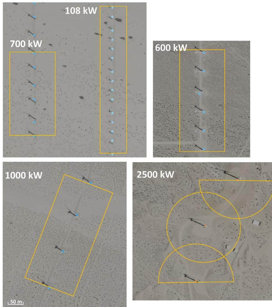
**FIGURE 1** San Gorgonio Pass Wind Resource Area located near Palm Springs, CA, USA. Sites are expanded to show search areas that extended 1.25x maximum blade height around turbines. kW indicates nameplate capacity of individual turbines in the string
