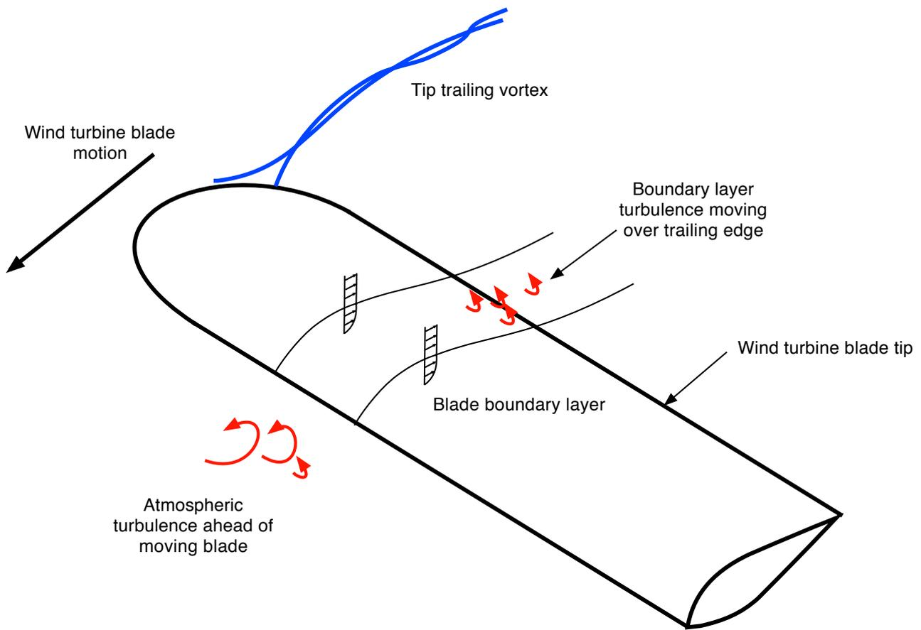
Figure 1: The flow over a wind turbine blade tip.
