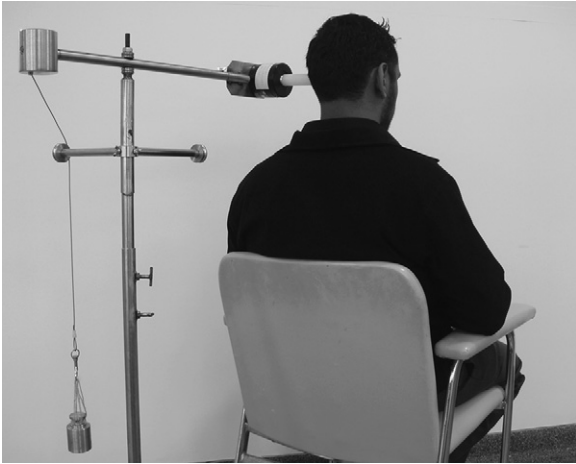
Fig. 1. A photograph of the experimental apparatus used to apply a perspex rod (attached to a B&K 4810 mini-shaker) with a constant tonic force to the mastoid of the subject. The stimulator is mounted on a 2:1 lever which can rotate freely in the horizontal plane and is pivoted on a vertical adjustable stand. A torque is applied at the opposite end of the lever by means of a mass M suspended by wire over a pulley below the fulcrum which can be adjusted so that the tension in the wire acts at an angle \theta to the plane of the lever. The tonic force at the mastoid then is given by F = 1/2 Mg \cos \theta , which for a mass of 1 kg and applied angle of 45^\circ is 3.5 N.
