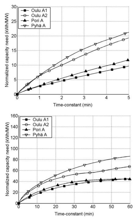
Figure 6a. Short-term influence of time constant  $\tau$  on the relative capacity need of the wind turbine storage unit. Turbine data sets with  $\Delta t = 1$  s and fluctuation class A
