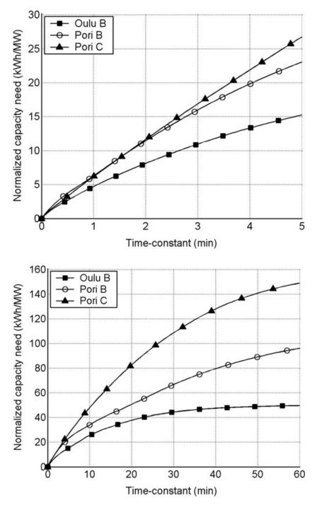
Figure 6b. Short-term influence of time constant  $\tau$  on the relative capacity need of the wind turbine storage unit. Turbine data sets with  $\Delta t = 1$  s and fluctuation classes B and C
