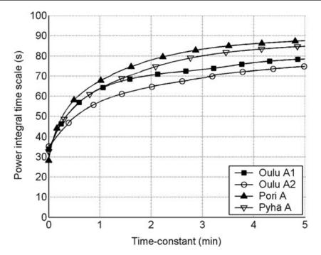
Figure 5a. Short-term influence of time constant  $\tau$  on the power integral time scale of the wind turbine power output. Turbine data sets with  $\Delta t = 1$  s and fluctuation class A
