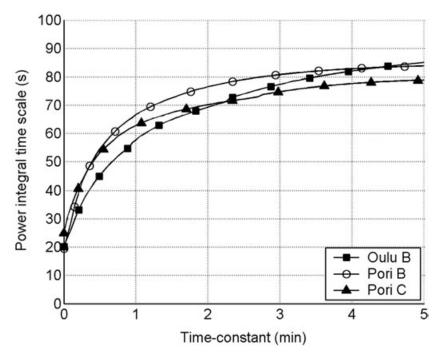
Figure 5b. Short-term influence of time constant  $\tau$  on the *r* power integral time scale of the wind turbine power output. Turbine data sets with  $\Delta t = 1$  s and fluctuation classes *B* and *C*
