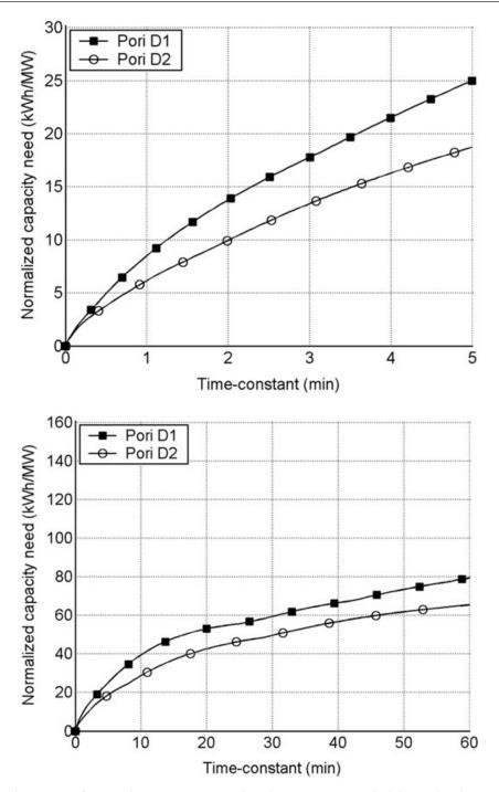
Figure 6c. Short-term influence of time constant  $\tau$  on the relative capacity need of the wind turbine storage unit. Turbine data sets with  $\Delta t = 1$  s and fluctuation class D
