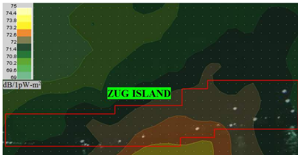
Figure 9: Contour Plot over Image from Pentangular Array – Measurement 1
