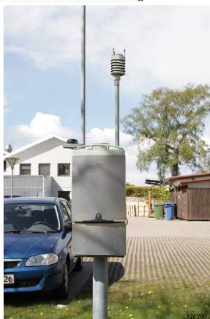
Fig. 2 Permanent NMT mounted on a pole (microphone on top of pole not visible)
