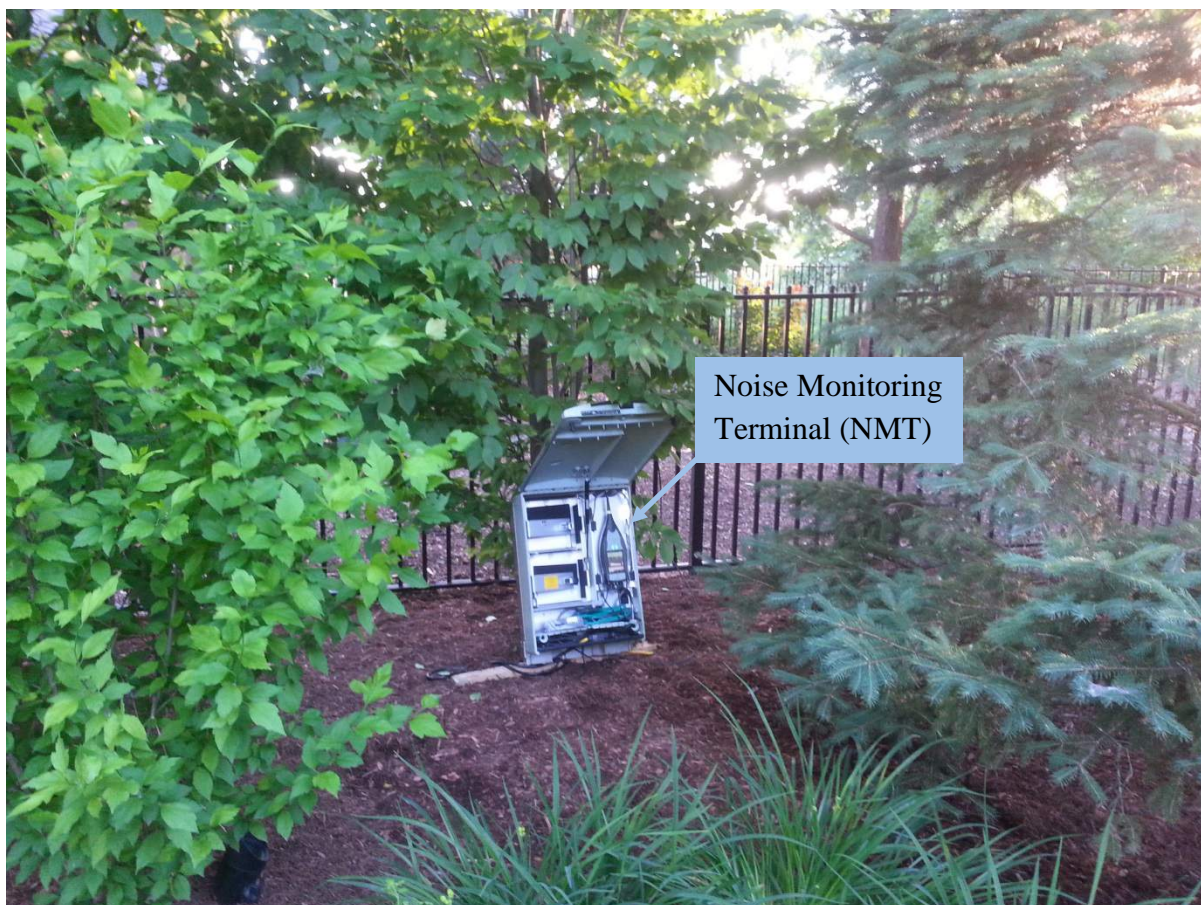
C 4: Installation of Portable Noise Sentinel at Local Residence – NMT
