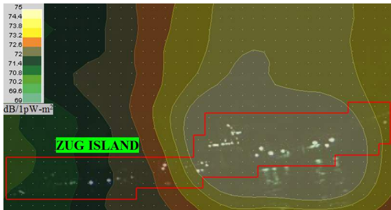
E 14: Contour Plot over Image from Pentangular Array – Measurement 5
