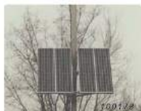
Fig. 9 Add solar panels to the NMT to reduce power consumption or even allow 24/7 battery operation
