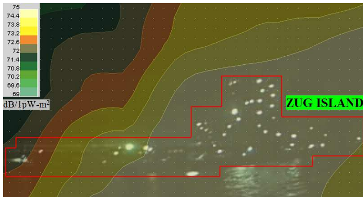
E 17: Contour Plot over Image from Pentangular Array – Measurement 6
