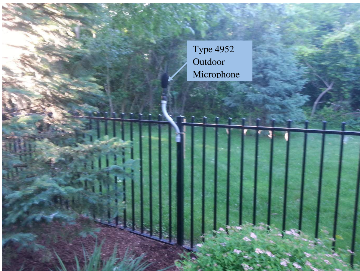
C 5: Installation of Portable Noise Sentinel at Local Residence – Microphone
