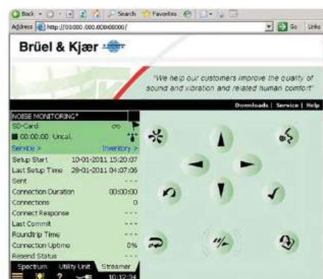
Fig. 7 View the results and status of the NMT remotely from a web browser
