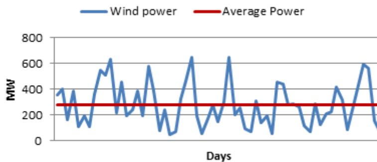
If we first make the assumption that the wind turbines owner want to sell an amount of energy equal to what its turbines will produce, that is to guarantee a power of 280 MW, the wind power will be used as follows without batteries:
