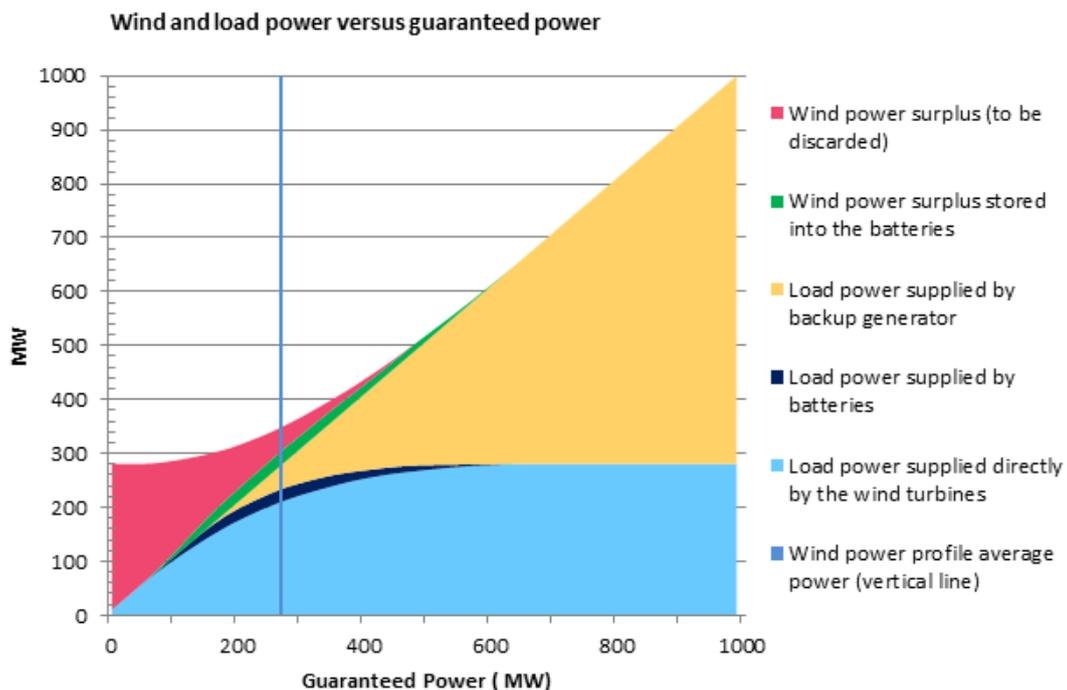
The figure is drawn for a 1000 MW power plant, with a wind load factor of 28%, coupled with backup power generators and 4GWh batteries. The values are calculated for each guaranteed power value based on the day by day simulation of the system. The resulting
