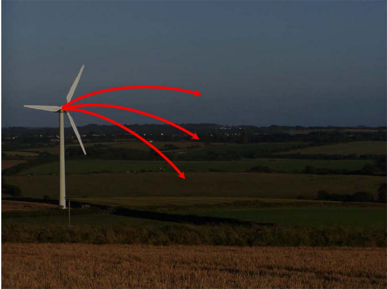
Figure 2. Sound rays curve downward towards the ground during the night. Sound rays also curve downward when sound propagates downwind.
