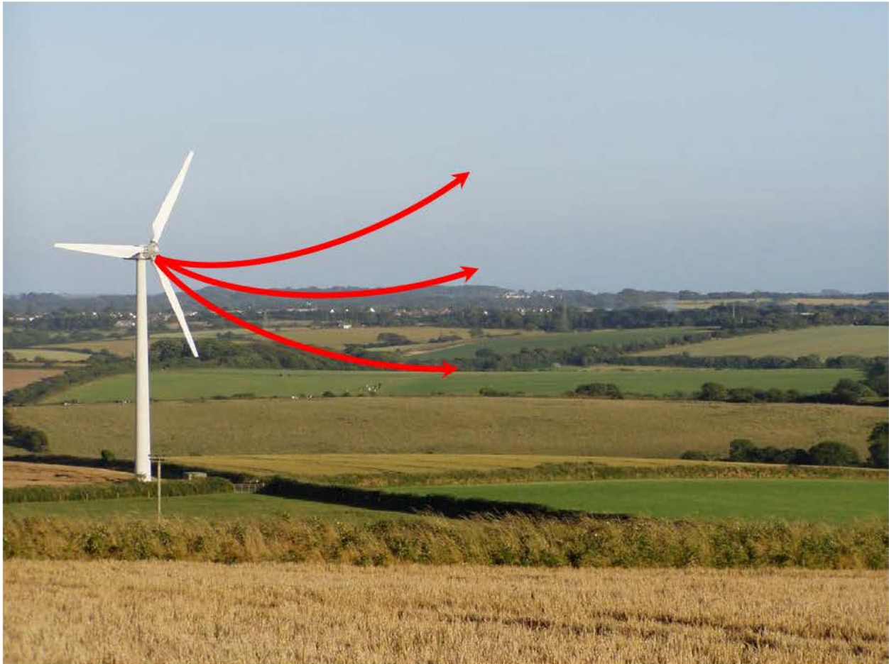
Figure 1. Sound rays curve upwards away from the ground during the day. Sound rays also curve upwards when sound propagates upwind.
