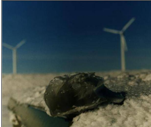
The picture at right is of a chunk of ice thrown hundreds of feet by a turbine.
