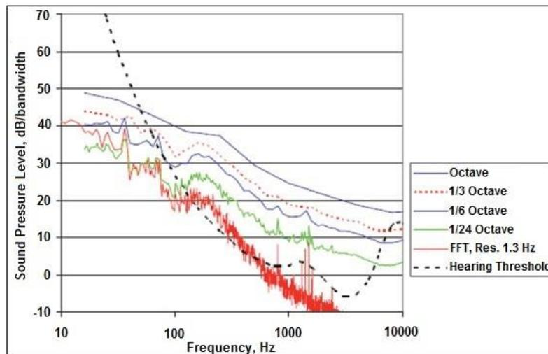
Figure 3. Different spectral analysis with the same signal of a wind turbine [29]
