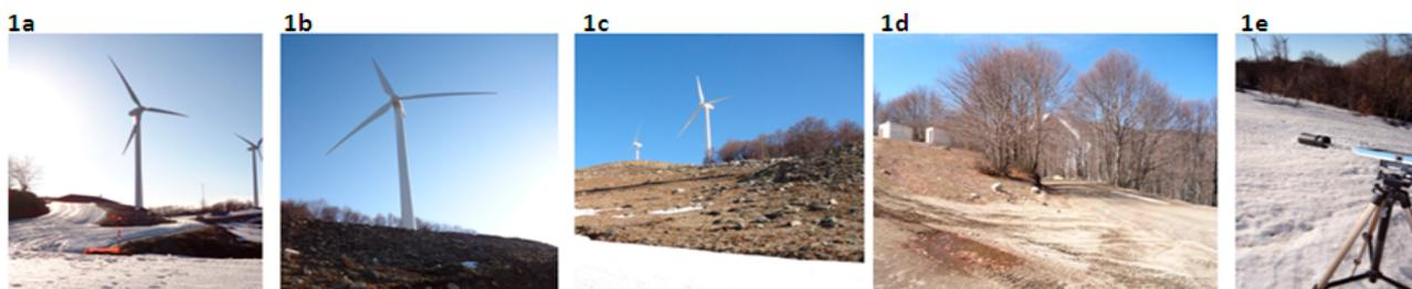
**Figure 1.** Pictures of the recording positions at: (a) 150 m; (b) 200 m; (c) 1500 m; (d) >2500 m. In (e) is shown the calibration of the sound level meter *in situ*.
