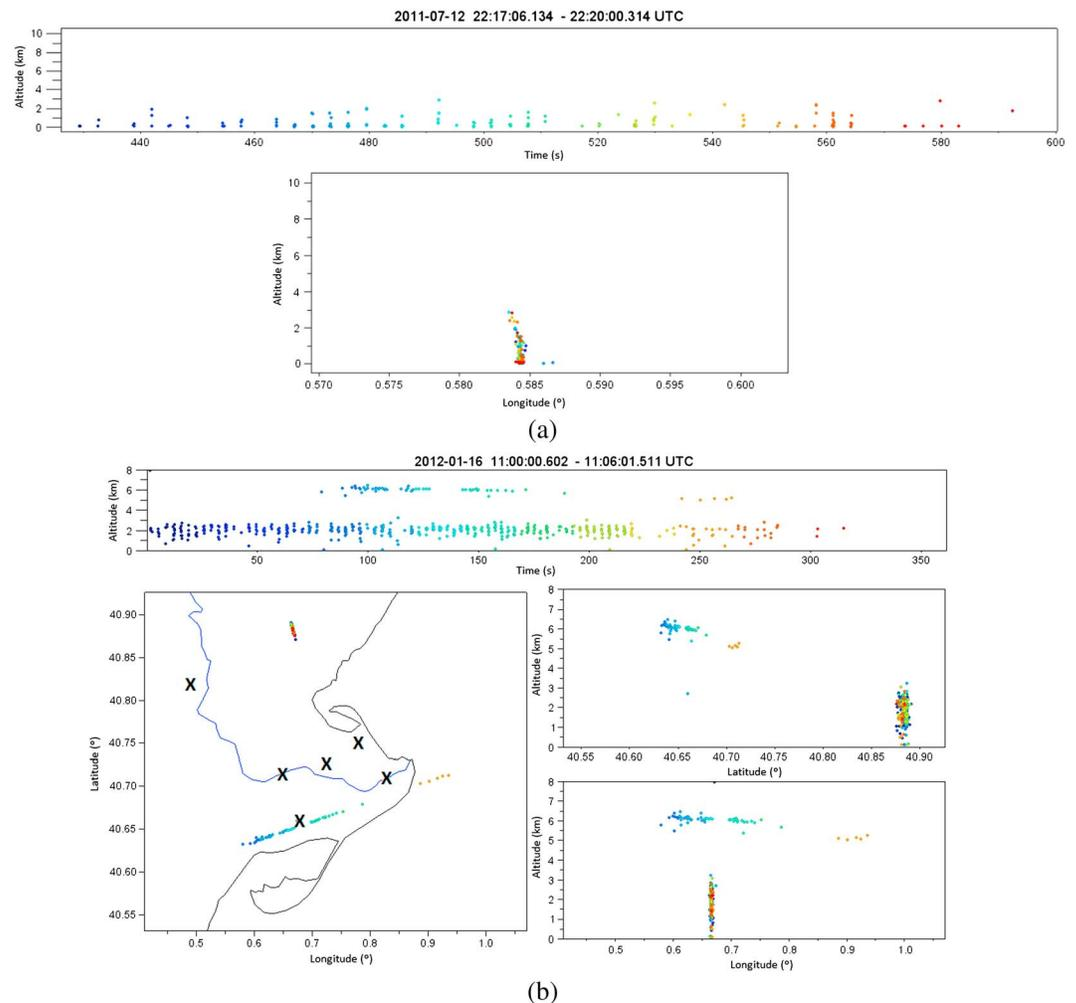
**Figure 2.** Two examples of repetitive detections of upward discharges from wind turbines. (a) Segment of about 3 min during 12 July 2011. (b) Segment of 10 min during 16 January 2012. In this period emissions produced by electric discharges in a plane were also detected (trace at ~6.5 km). The (cross) symbols in the plan view indicate the locations of the ELMA stations.
