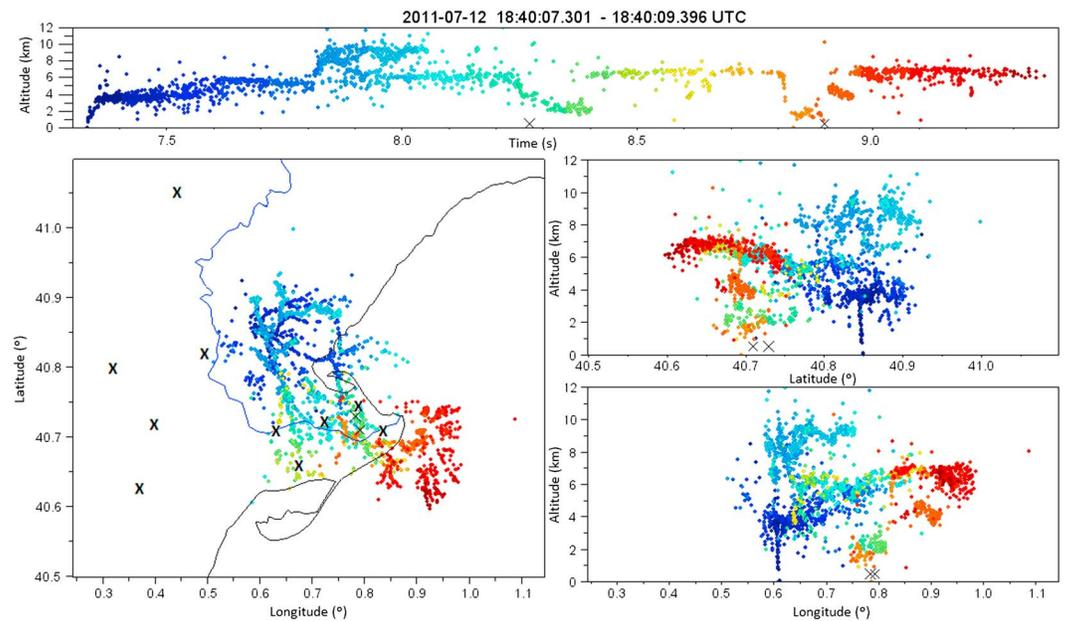
**Figure 3.** ELMA sources of the upward flash on 12 July 2011 originating on a wind turbine and terminating at ground. The (cross) symbols in all the views indicate ground strokes detected by LINET VLF/LF network [Betz *et al.*, 2004]. The (cross) symbols in the plan view indicate the locations of the ELMA stations.
