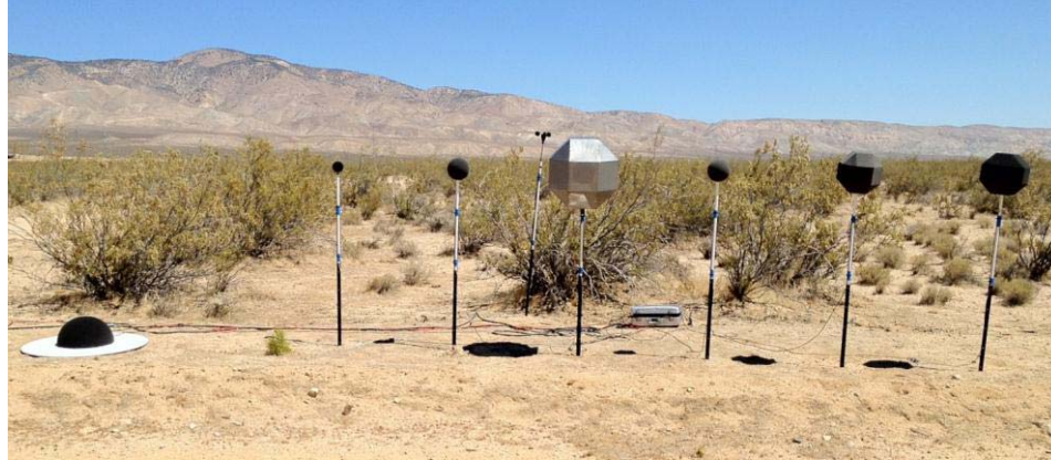
FIGURE 3. Comparative windscreen test setup in the Mojave Desert.
