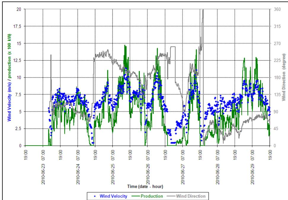
FIGURE 3: Parameters measured at the Hub of a wind turbine, June 22<sup>nd</sup> to June 29<sup>th</sup>, 2010.
