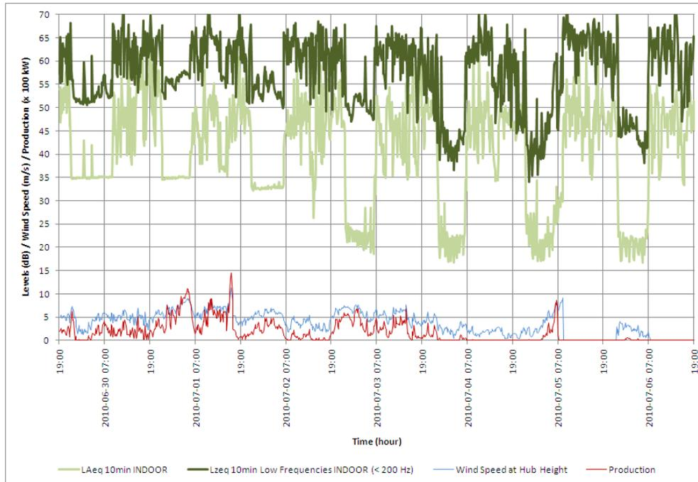
**FIGURE 6: Noise levels measured indoor of a residence,  $L_{eq}$  10min, June 29<sup>nd</sup> to July 6<sup>th</sup>, 2010.**
