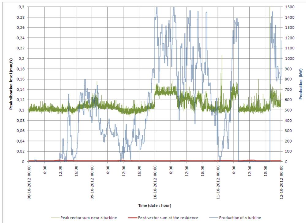
FIGURE 7: Ground vibration levels measured, October 8<sup>th</sup> to October 12<sup>th</sup>, 2012.
