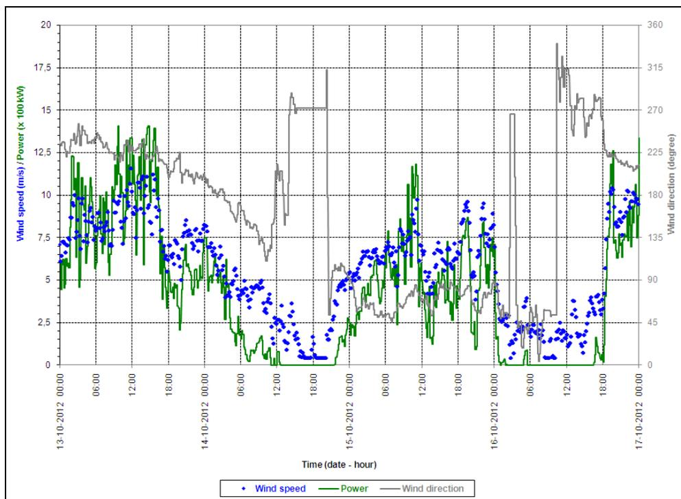
FIGURE 1: Parameters measured at the hub of a wind turbine, October 13<sup>th</sup> to October 17<sup>th</sup>, 2012.
