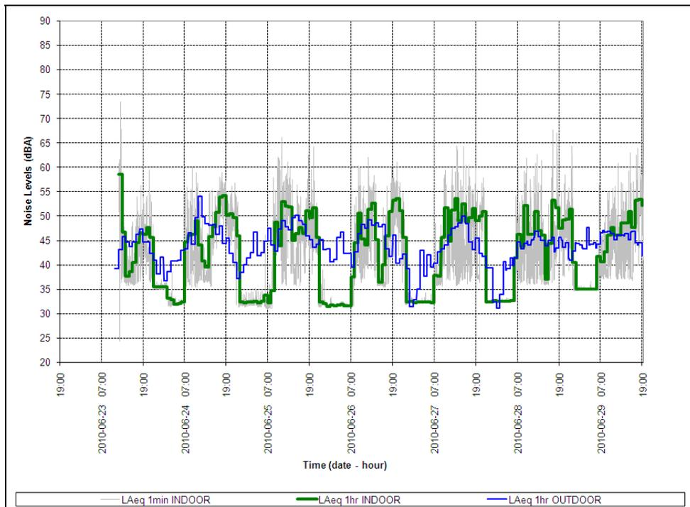
FIGURE 4: Noise levels measured outdoor and indoor of a residence,  $L_{Aeq}$  1hr, June 22<sup>nd</sup> to June 29<sup>th</sup>, 2010.
