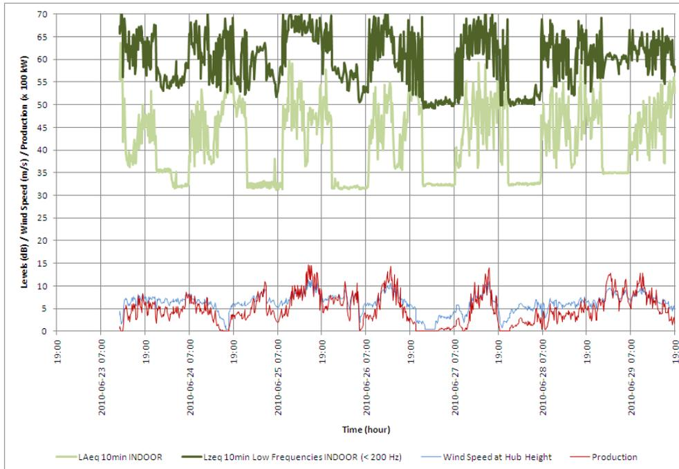
**FIGURE 5: Noise levels measured indoor of a residence,  $L_{eq}$  10 min, June 22<sup>nd</sup> to June 29<sup>th</sup>, 2010.**
