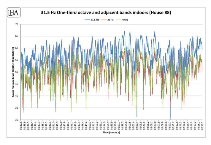
Steven, you will see that the proposed acceptable sound level (56 dB) in the 31.5 Hz one-third octave band is exceeded by up to 10 dB.
