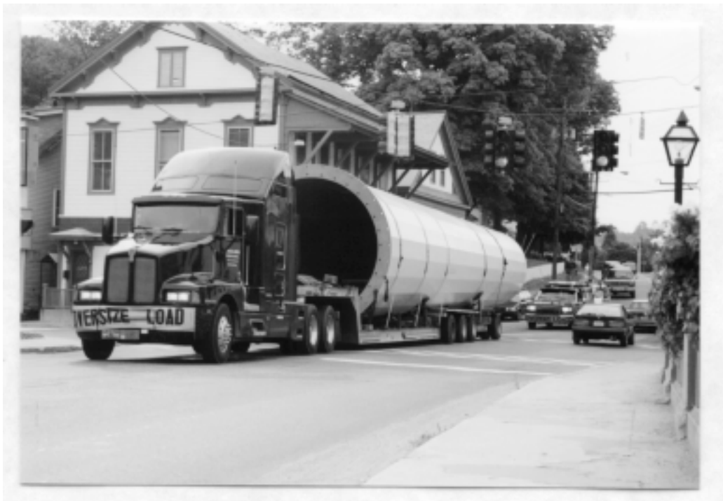
Figure 10-1 A Bottom Tower Section Moving Through the Town of Wilmington, Vermont
