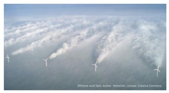
So a wind wake is something that a utility-scale wind turbine creates. Typically 'wind wake' refers to a long trail of turbulent wind behind the turbine that has diminishing speed and energy content. Once wind has flowed through a wind turbine, the air downstream of that turbine has reduced wind speed and increased turbulence, compared with wind flowing in the free stream before it interacts with that wind turbine. These wakes, like ships' wakes, rotate in a corkscrew-like pattern.
