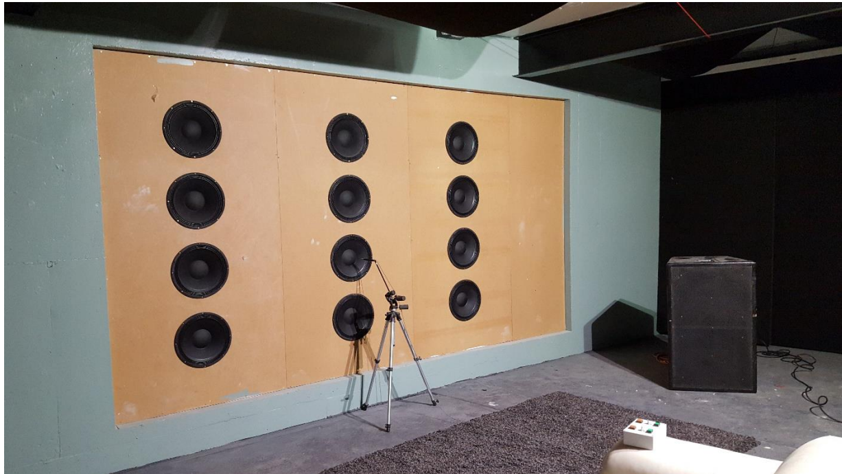
Figure 5: Speakers in 10.5 m 2 opening to 126m 2 reverberation room
