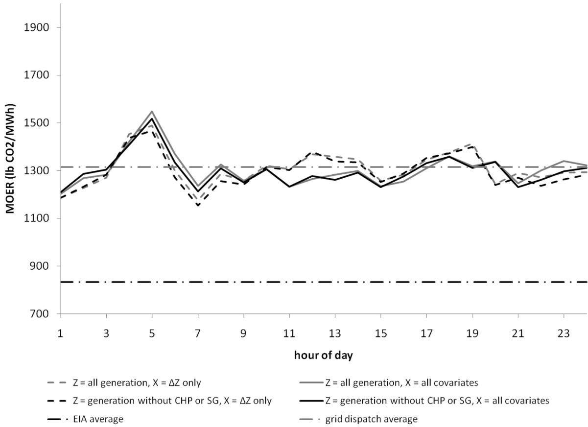
Figure 5a: Marginal operating emissions rates for ISONE
