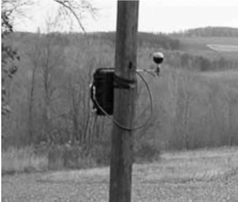
Fig. 2: Hessler's Typical Background Sound Measurement Setup (Brown Hill, Loc. 2)
