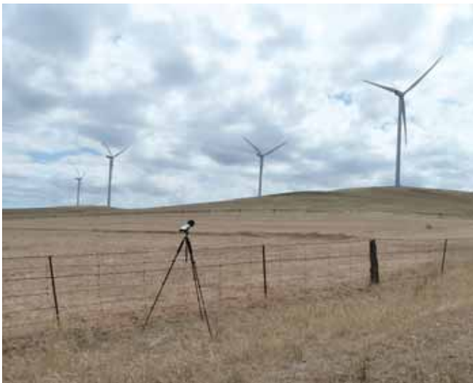
Figure 3. Monitoring wind turbine noise at an operating wind farm, Waterloo, South Australia. Notice that the blades of the four turbines have closely matched phase. Considered as a random event, the chance of 4 turbines having all phases equal to within 5^\circ of each other are (5/360)^3 = about 1 in 2 million. Photo: EPA South Australia, with permission.
