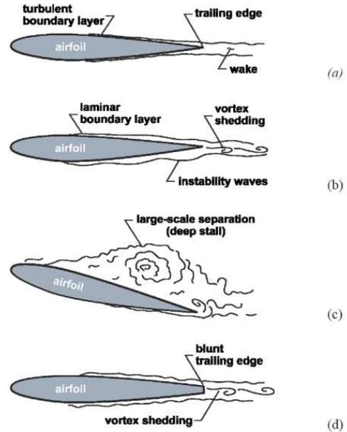
Figure 10: Airfoil Self-Noise Mechanisms (Oerlemans (2011))
