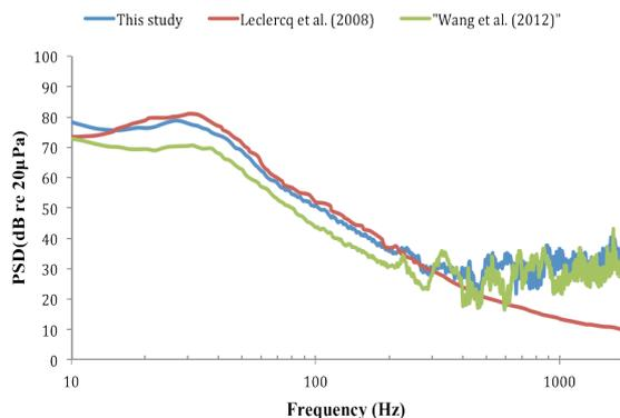
**Figure 13.** Comparison of estimated wind noise spectra with Wang, Zander and Lenchine (2012) and Leclercq, Cooper and Stead (2008) at airflow velocity of 8 m/s and for 90 mm windshield
