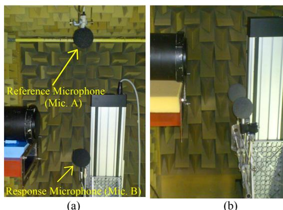
**Figure 1.** Experimental arrangements, (a) Arrangement 1, both microphones equipped with a 90 mm windshield and (b) Arrangement 2, both microphones equipped with a 75 mm windshield
