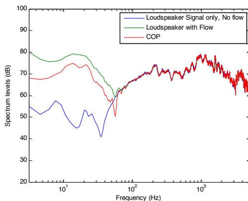
**Figure 17.** Auto spectra of a microphone in Arrangement 2 located in the jet with loudspeaker signal, with and without flow, as well as the COP spectrum between the microphones in Arrangement 2 for a 45 mm windshield and airflow velocity of 4 m/s
