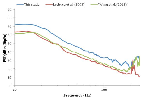
**Figure 12.** Comparison of estimated wind noise spectra with Wang, Zander and Lenchine (2012) and Leclercq, Cooper and Stead (2008) at airflow velocity of 4 m/s and for 90 mm windshield
