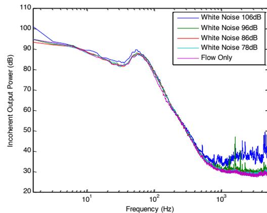
**Figure 8.** IOP between microphones positioned in Arrangement 1 and equipped with 60 mm windshields at airflow velocity of 16 m/s and different loudspeaker levels
