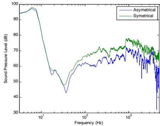
**Figure 11.** Autospectra of reference microphone for Arrangement 1 equipped with 45 mm windshield with airflow velocity of 16 m/s for symmetrical and asymmetrical positioning of microphones
