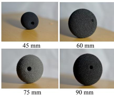
**Figure 3.** Different windshields used in experiments
