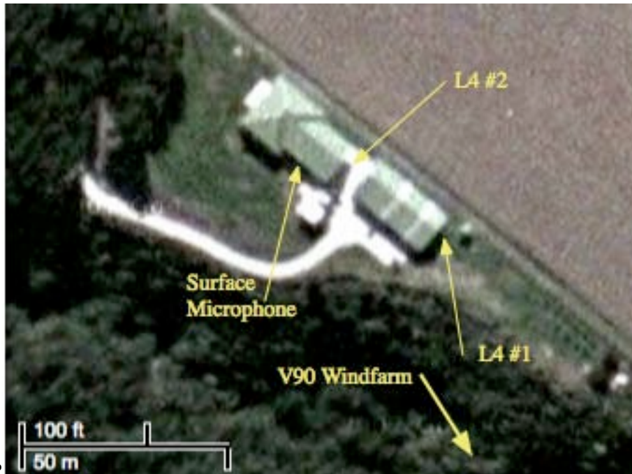
Figure 1: Site layout and position of sensors. (© Copyright 2009 Google Map Data)
