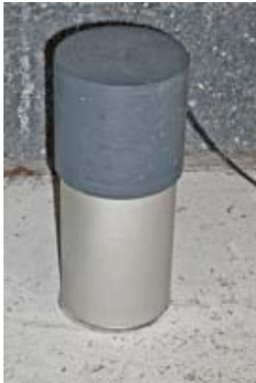
Figure 3: Photo of L4 geophones in situ; bonded to the carport floor and buried in the ground.
