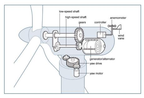
Behind the blades, a low-speed shaft transfers the rotational force of the rotor to the gearbox. The gears of the gearbox were machined using precision tools and special hardened steel components. The gears increase the low rotational speed of the rotor shaft to the high speed needed to drive the generator.
