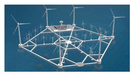
The turbines can be replaced while the steel platform itself should last for 50 years or more.
