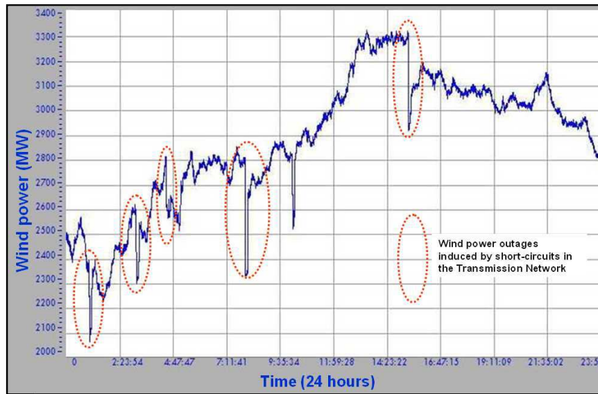
Figure 4.a.- Recorded wind power and wind power outages induced by well cleared short-circuits in the Transmission Network (Spain).
