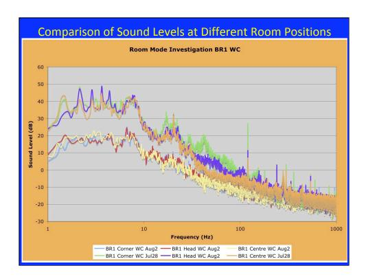
Here we see the FFT display of the sound levels for frequencies between 1 and 1000 Hz at the three monitoring locations in BR1 - centre of room, head of bed = middle of wall, and corner of the room, on two separate dates, when the turbines are not operating (on August 2nd) and when turbines are at moderately high power (on July 28<sup>th</sup>). Note that these readings were performed with all windows closed, on this solid home with casement windows including tight seals.
