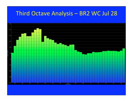
Wrapping up, one particular factor that was noticed when watching the real time third octave analysis of the conditions inside the rooms of the study home, was the amplitude variation in each frequency allocation.
