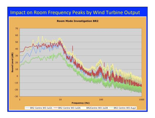
In this chart only the centre of the room data is shown, for 4 different cases to show the comparison of room mode values with no turbines, and with turbines operating at powers of 0% / 30% / 65%
