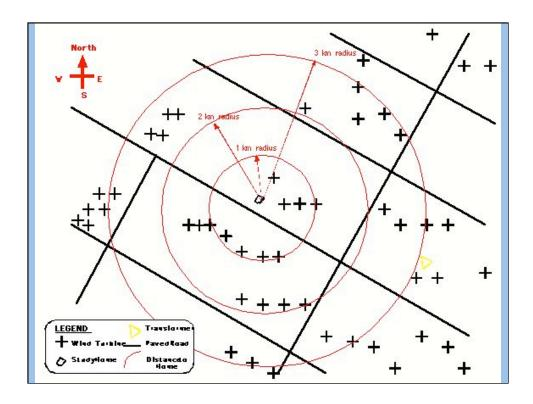
This drawing shows the study home surroundings, typical of others approved by the Ontario Ministry of the Environment. The home has 9-1.65 MW wind turbines with 82 metre rotors on 80 metre hub height towers within 1000 metres, 6 more turbines from 1000 metres to 2000 metres, and 17 more turbines from 2000 metres to 3000 metres. The substation and step up transformers of the array are located just over 3000 metres from the home.
