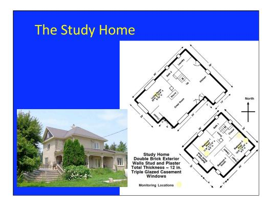
The study home where recordings were permitted (any hour of he day or night) is typical of a century Ontario Farmhouse, but with extensive upgrades. The home exterior walls are a double brick construction. Interior insulation, and a lath and plaster wall, in some cases with a further interior gypsum wallboard construction result in an overall wall thickness of some 12 inches (30 cm). Windows are upgraded modern design with triple glazed casement construction, and resilient gasket seals.
