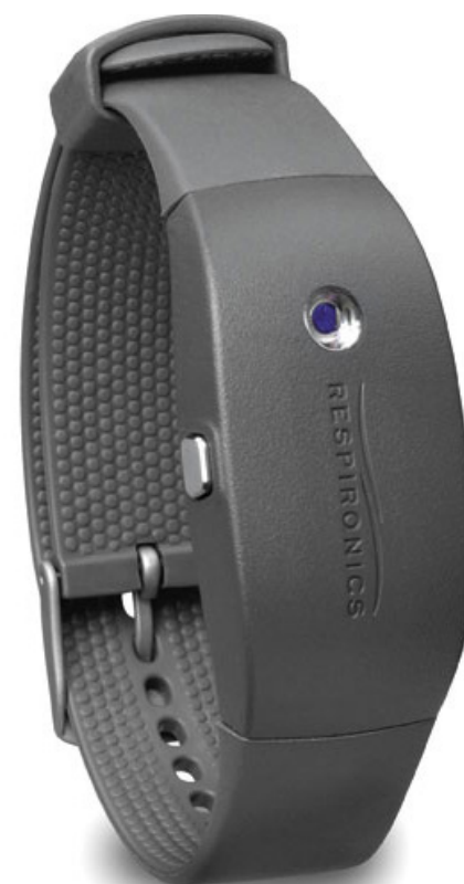
The Actiwatch 2 is used to provide measures of sleep onset, total sleep time, awakenings, and sleep efficiency.
