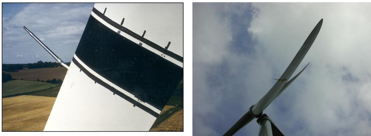
Figure 1 In the left figure is shown the first use in 1987 of the five hole pitot tube on a 19m diameter rotor. To the right, the same tube was mounted at radius 26.2m (66% radius) on the 80m rotor for the campaign in 2003 in the Tjaereborg wind farm. These data are used for the analysis in the present paper.
